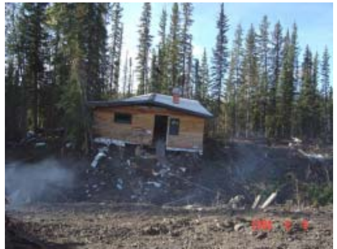
Above: The water and ice had receded by summer, but the destruction of many homes, moved right off of their original foundations, was still evident.
